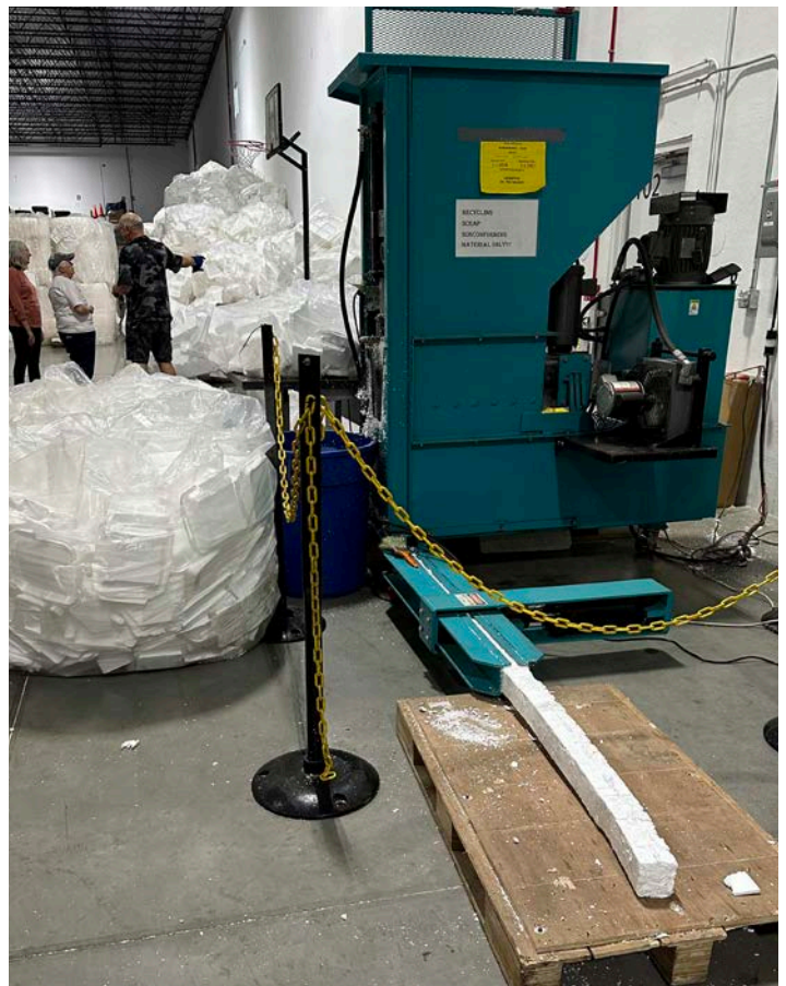
Densifier to transform Styrofoam into 2x4 logs
